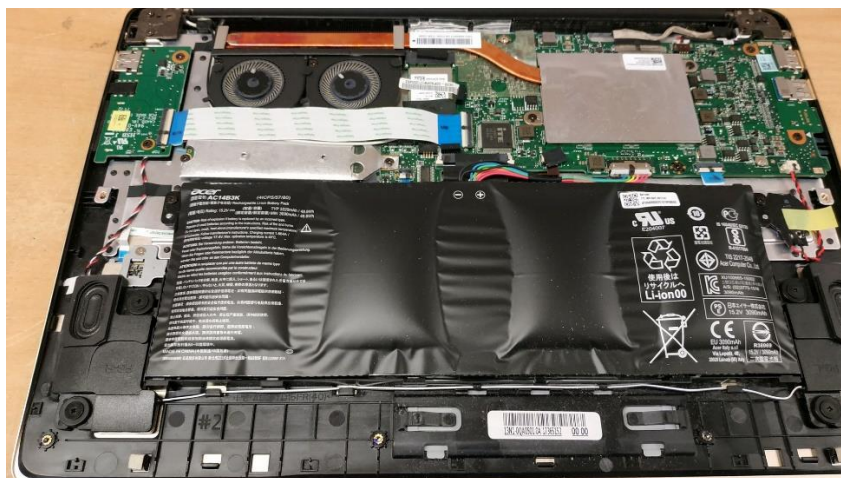
Faulty and swollen Li-ion batteries on a laptop (Credit: www.assistancepc.fr )
